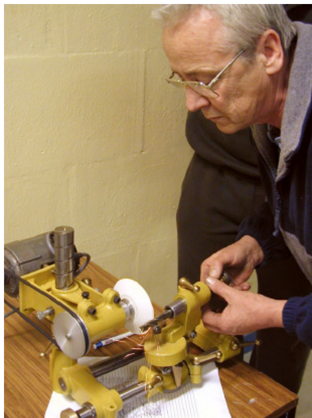
Phil Gibbons demonstrates the use of his Quorn Tool & Cutter Grinder at the July Meeting.
