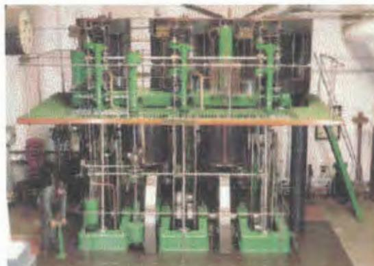
**Photo 1** – Hathorn Davey Triple Expansion Engine c.1910
