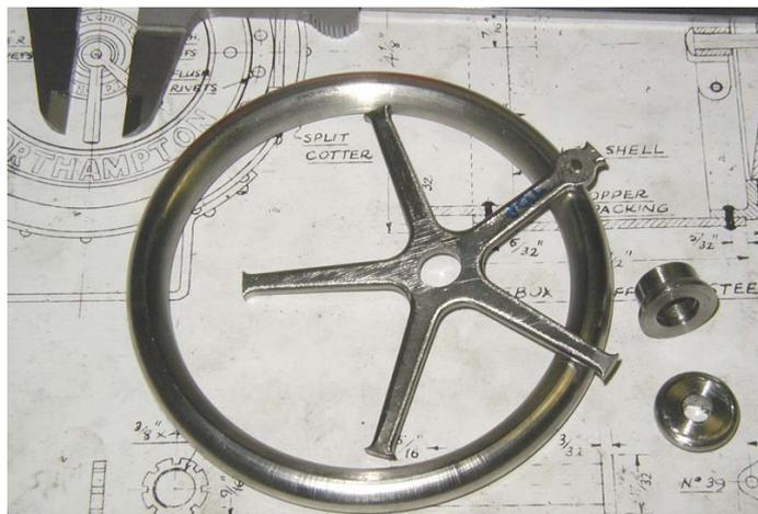
Above: Components to make an Allchin steering wheel. The central spider is laser cut, the outer ring and bushes are machined from stainless, then it's all silver brazed together. Photo: Jim Clark
