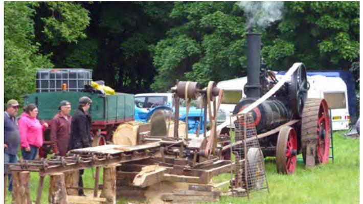
Doing what it was built to do: A Wm Foster and Co steam traction engine powering a timber saw (where was Health and Safety?).
