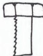
Left-hand thread (right-hand version also available)
