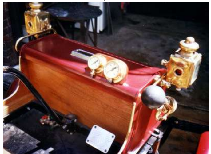
Driver's eye view of controls and gauges. Note the authentic brass lamps, originally from a London cab. Photos: Stu Martyn
