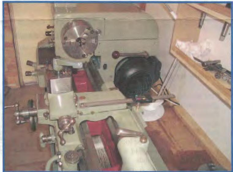
Digital readout. Transducers that I have dealt with in the past used some form of mechanical interface, usually in the form of a slotted wheel or similar. My concern was that with the constant use, the thing would wear and create substantial errors.
