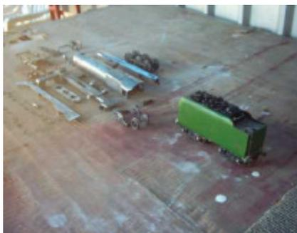
The next few pics show the progress to date of how far I've managed to get. With the loco fully stripped down to just bare metal, I had a lot of work ahead of me to disassemble the loco into each part and clean up ALL the bad castings as they had a lot of "pitting" from being left in a damp environment – but being mostly made of Aluminium as I discovered – there was a lot of flashing from the casting process that still needed to be filed off
